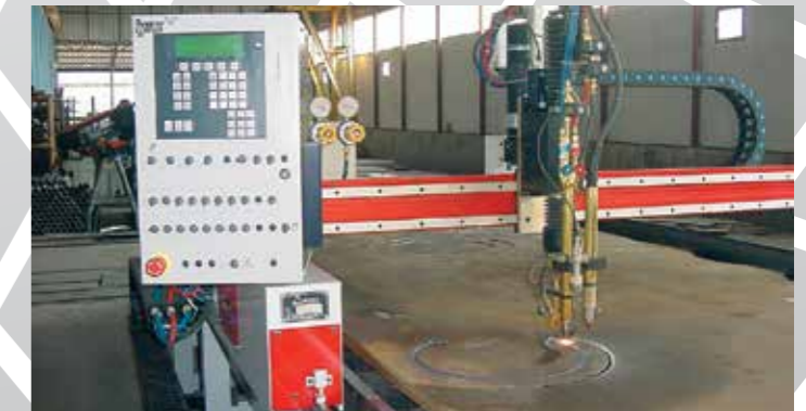
CNC Plazma Kesme Makinesi (3000 x 15.000 mm) CNC Plasma Cutting Machine (3000 x 15.000 mm)
