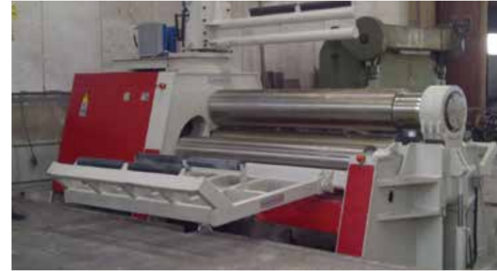
4 Top Silindir / 4 Roll Bending Machine (50x3000 mm)
